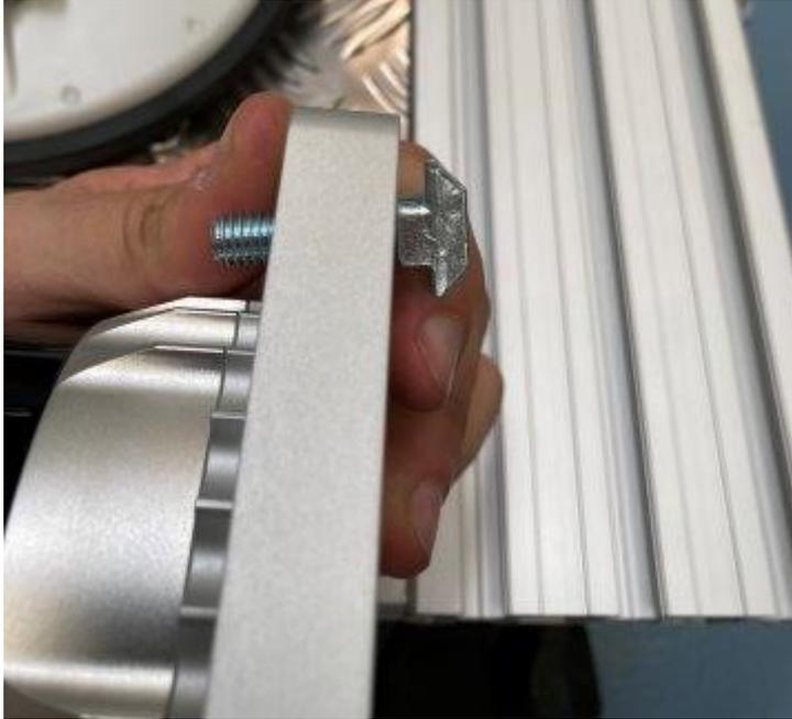
+ PRO TIP: Screw the M8 flange nuts loosely. That will help with the alignment of the T-head bolts and the grooves on the side decks.
