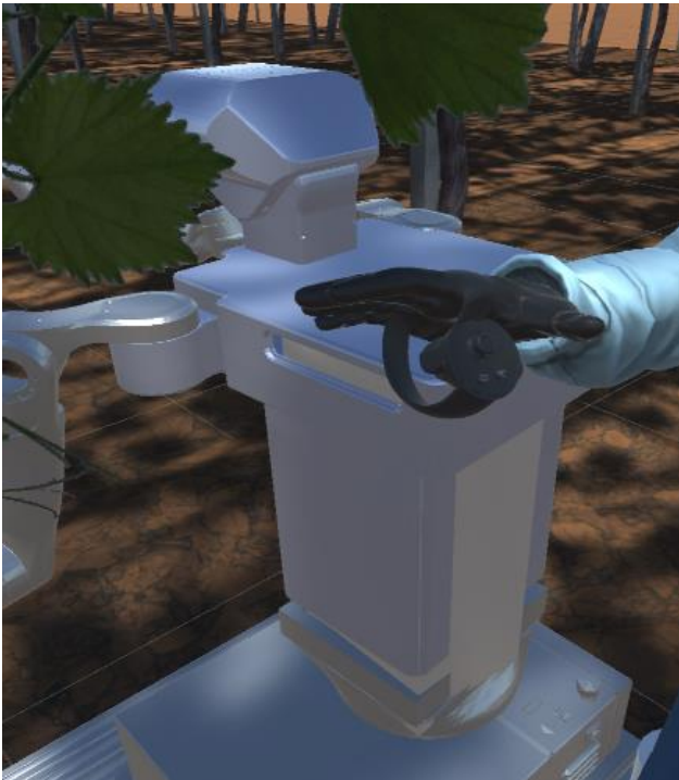
Figure 3 Human hand without collision: the controller is located in the hand palm.
