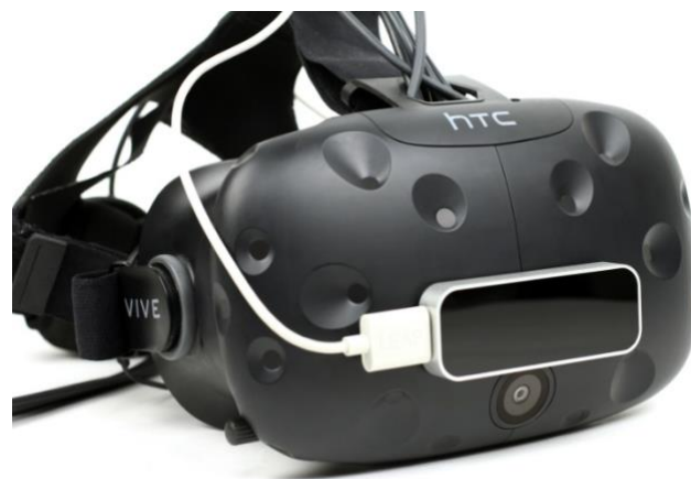
Figure 6 HTC Vive with Leap Motion hand tracking device attached
